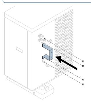
Install the gas separator (HN1) on the upper 90-degree coupling and the check valve (XX#) on the lower 90degree coupling.
