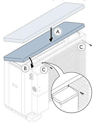
**15.** Attach the cover for the safety valve (FL2) to the gas separator casing.
