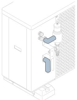
**8.** Install the rear and front insulation blocks around the gas separator.
