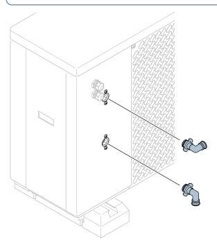
2. Ensure that the 90-degree coupling are mounted so that the coupling for the heating medium supply (XL7) points to the right and that the coupling for the heating medium return (XL8) points downwards.
