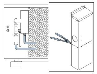
If the pipes are mounted vertically, the gas separator casing does not need to be modified.
