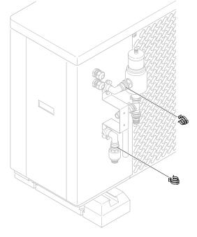
7. Attach condensation insulation along the pipes, from the back of the heat pump to the gas separator and over the check valve.
