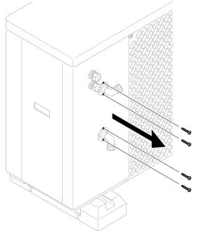
**4.** Fasten the 90-degree couplings and the supplied bracket with the supplied hexagonal screws.
